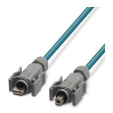
Assembled USB cable, shielded, color: RAL 5021 (water blue), PUR outer sheath, USB type A/IP67 on USB type B/IP67, length: 2 m
